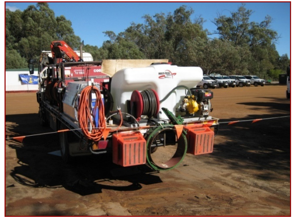
Fire-fighting equipment on welding truck
