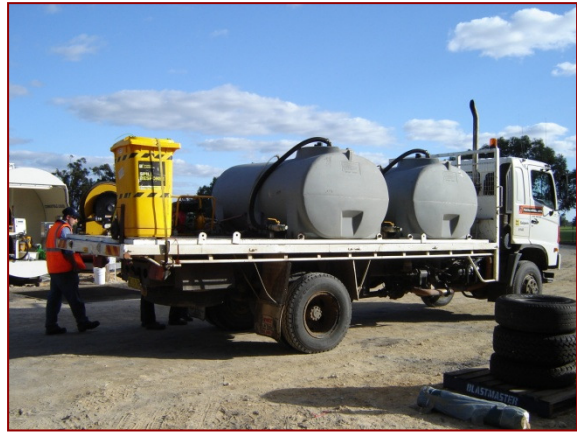
Spill cleanup kit on rear of fuel truck
