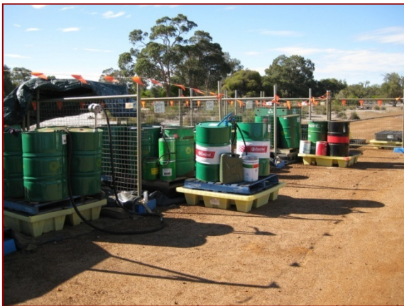
Bunded storage of oils in fenced and signposted areas
