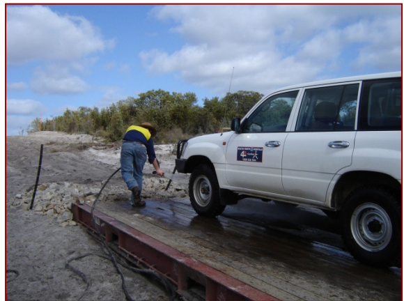
Vehicle washdown hygiene facility at entry to Bush Forever site
