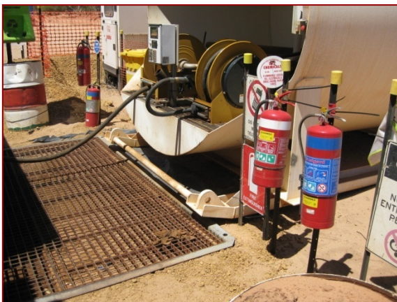
Refuelling grate, spill kits and fire control measures at bulk refuelling station
